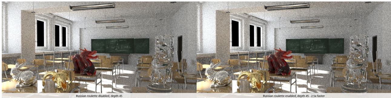
Figure 16: Using Russian roulette for early path termination can significantly reduce render times, with a small increase in variance.
